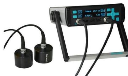
Gambar 1. Alat *Ultrasonic Pulse Velocity* (UPV)
