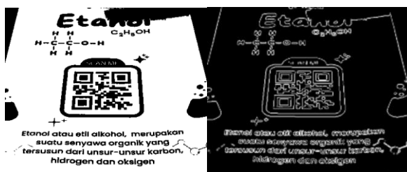
Gambar 3. Contours Extraction dan Corner Detection Figure 3. Contour Extraction and Corner Detection
