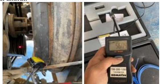
Gambar 9. Pemasangan stiker dan laser tachometer Figure 9. Installation of Sticker and Laser Tachometer
