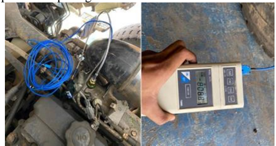
Gambar 8. Pemasangan alat thermocouple Figure 8. Thermocouple Installation
