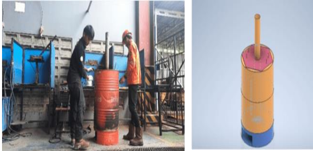
Gambar 1. Alat tungku materail drum Figure 1. Material drum Furnace Tool
