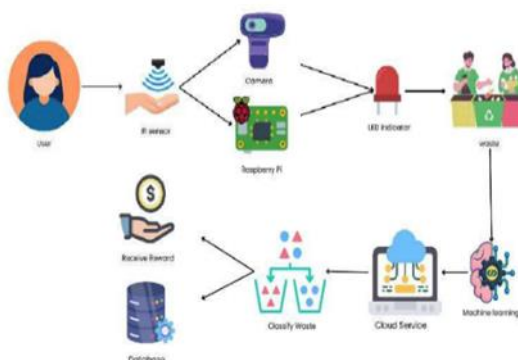
Gambar 6. Arsitektur Sistem BINSIGHT Figure 6. BINSIGHT's System Architecture
